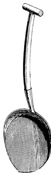
Fig. 252. — Frying-pan or lime shovel.
