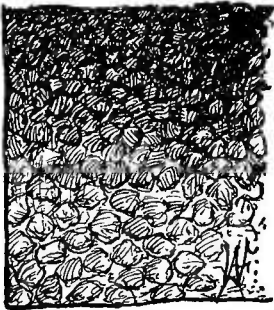
Fig. 28. Showing the effect of the roller in compacting the surface layer.
